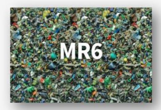
MR6 IS MANUFACTURED FROM A MIX OF RECYCLED POLYMERS, DESIGNED TO MODIFY ASPHALT AND REDUCE DEFORMATION FAILURES OR INCREASE STIFFNESS.
